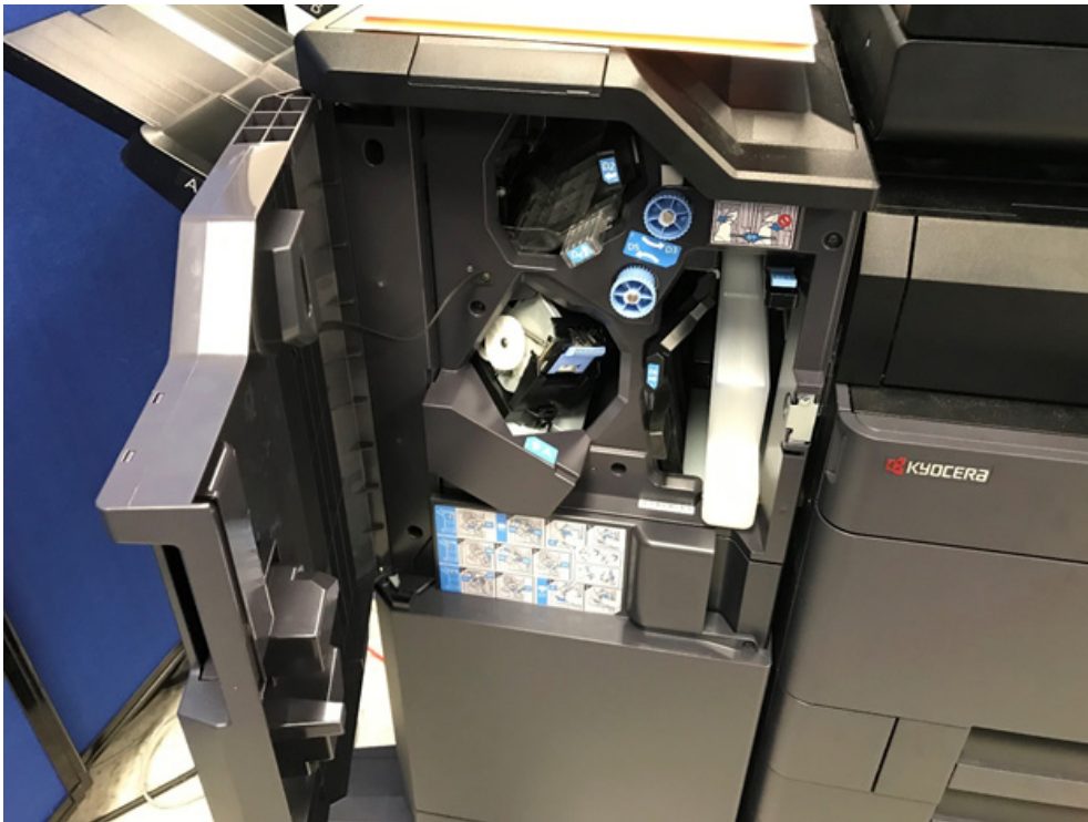
Misfeed areas are easily identified inside the machine with blue labels and numbers.
