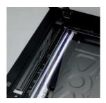
LED scanner uses less energy than conventional lamps.
